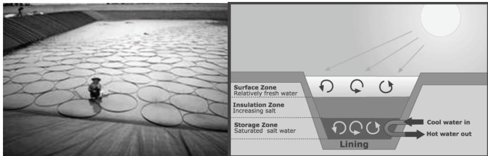
Fig. 2a. (Left) Solar pond for heating purpose demonstration in Australia ( http://www.aph.gov.au/library/pubs/bn/sci/RenewableEnergy_4.jpg ). 2b. (Right) Solar Ponds Schematic The salt content of the pond increases from top to bottom. Water in the storage zone is extremely salty. As solar radiation is absorbed the water in the gradient zone cannot rise, because the surface-zone water above it contains less salt and therefore is less dense. Similarly, cooler water cannot sink, because the water below it has a higher salt content and is denser. Hot water in the storage zone is piped to, for example, a boiler where it is heated further to produce steam, which drives a turbine. (Wright, 1982; and www.energyeducation.tx.gov/.../index.html )
